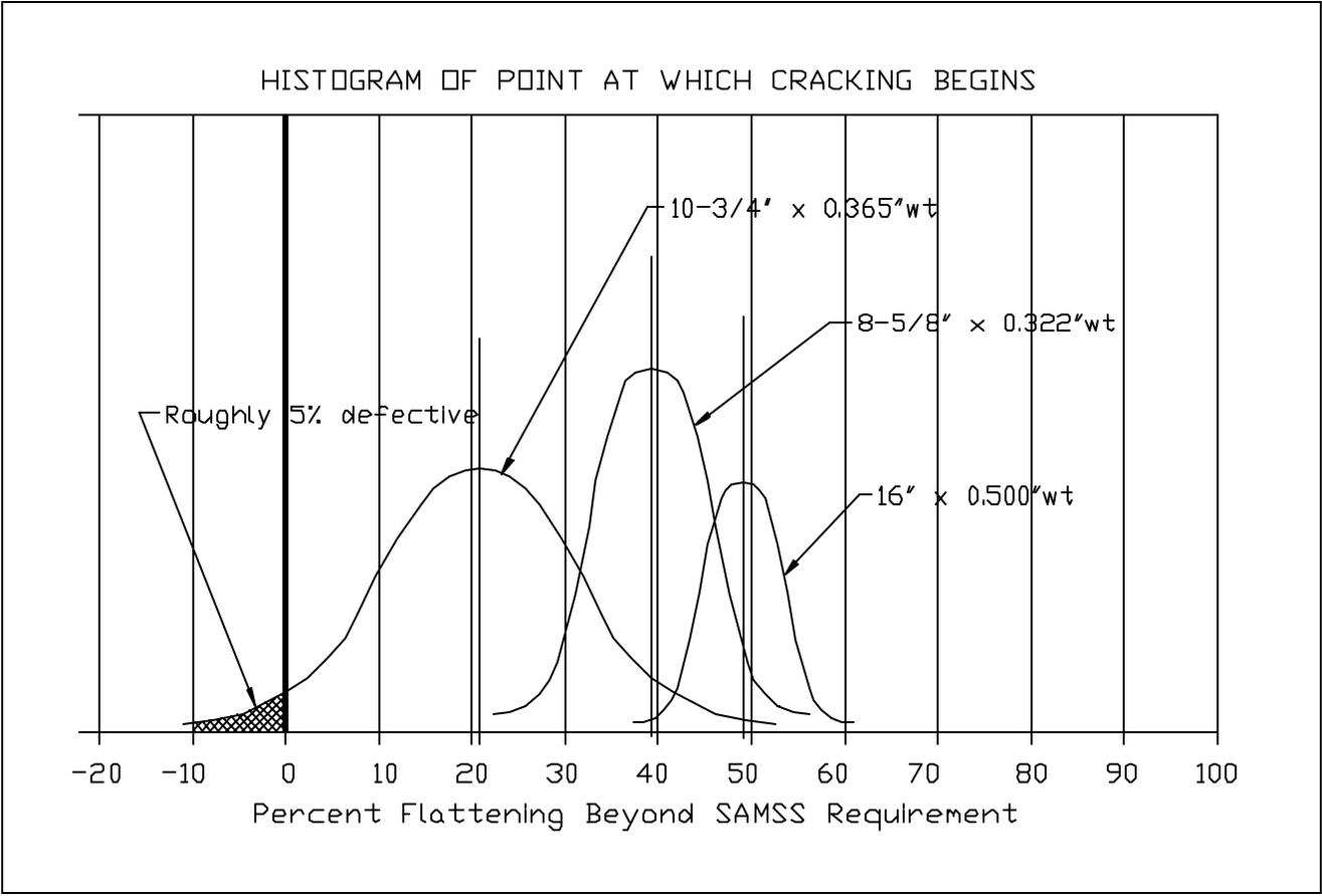
Figure 18 - Chart showing actual production performance of three pipe sizes during flattening test. Pipe mill must maintain a standard deviation of 3.0 maximum during qualification so that the production average of flattening tests will exceed 20% beyond the minimum flattening height.
