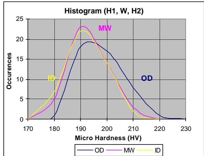
Figure 13 - Micro-hardness variation measured on regular production samples
