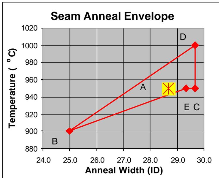
Figure 11 - Qualification boundary chart produced by software using actual production data
