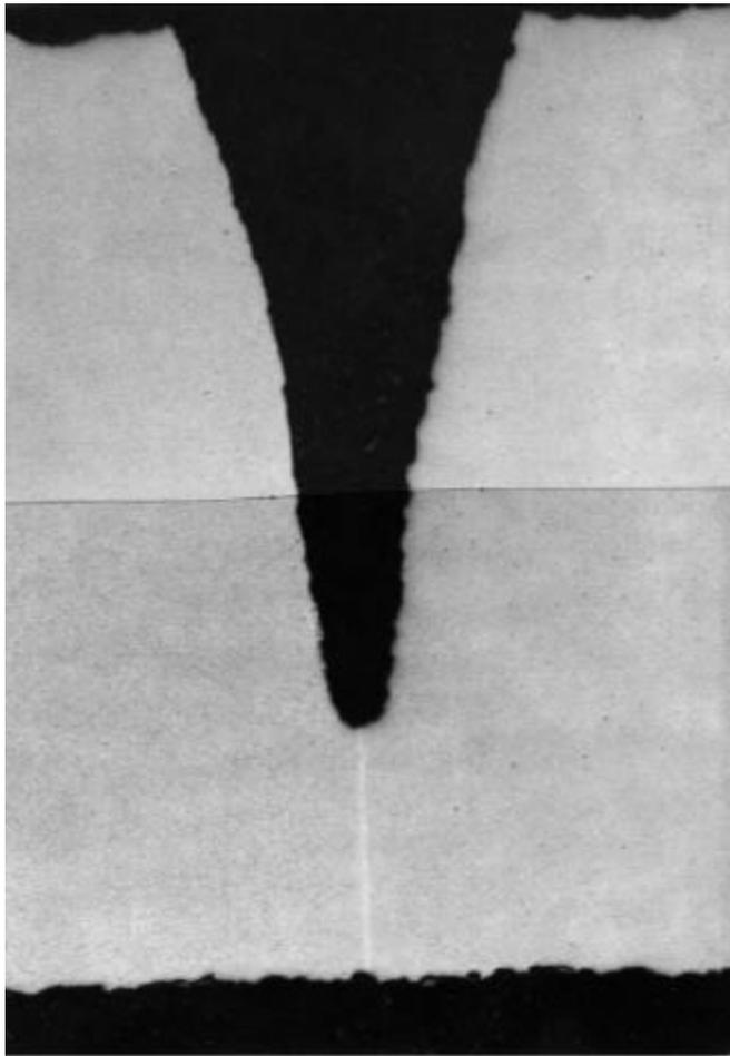
Figure 3 - API 5L Gr B 12 inch OD and 0.375 inch WT, produced prior to 1981, which failed due to grooving corrosion of the ERW weld seam
