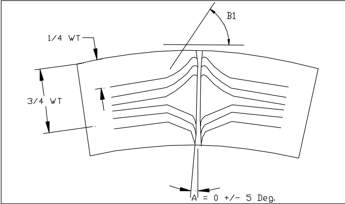
Figure 8 - Metal distortion angle measurement location
