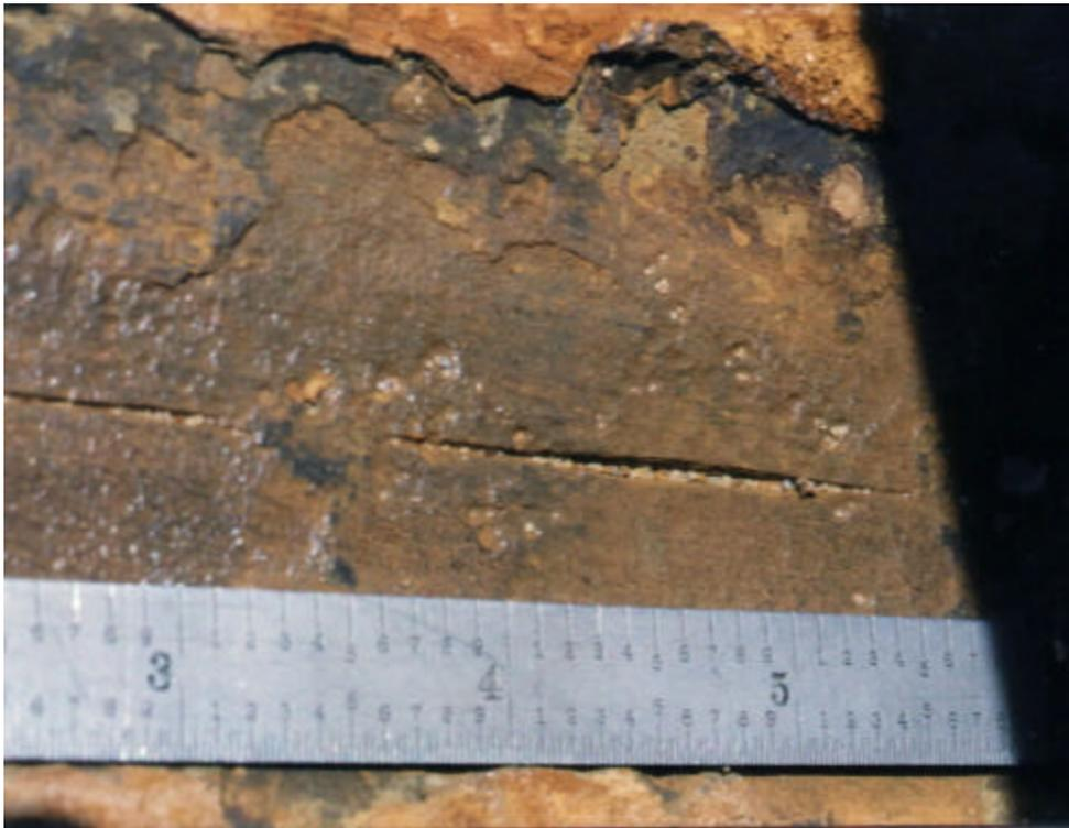
Figure 4 - API 5L Gr B 12 inch OD and 0.375 inch WT, produced prior to 1981, exhibiting varying degrees of grooving corrosion.
