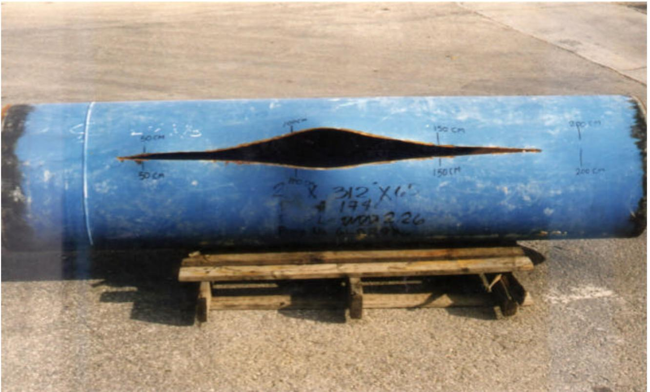
Figure 2 - API 5L X65 20 inch OD and 0.312 inch wall thickness which failed during field hydro-test
