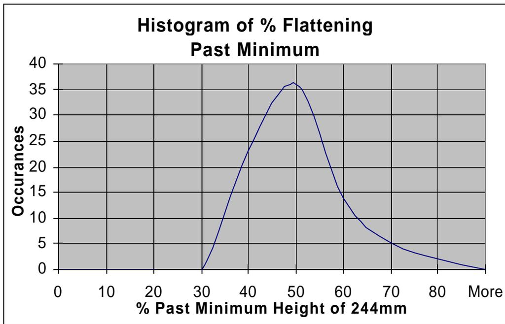
Figure 17 - Actual performance of production flattening tests continuing beyond minimum flattening height until splitting failure occurs (See Figures 16 & 18).
