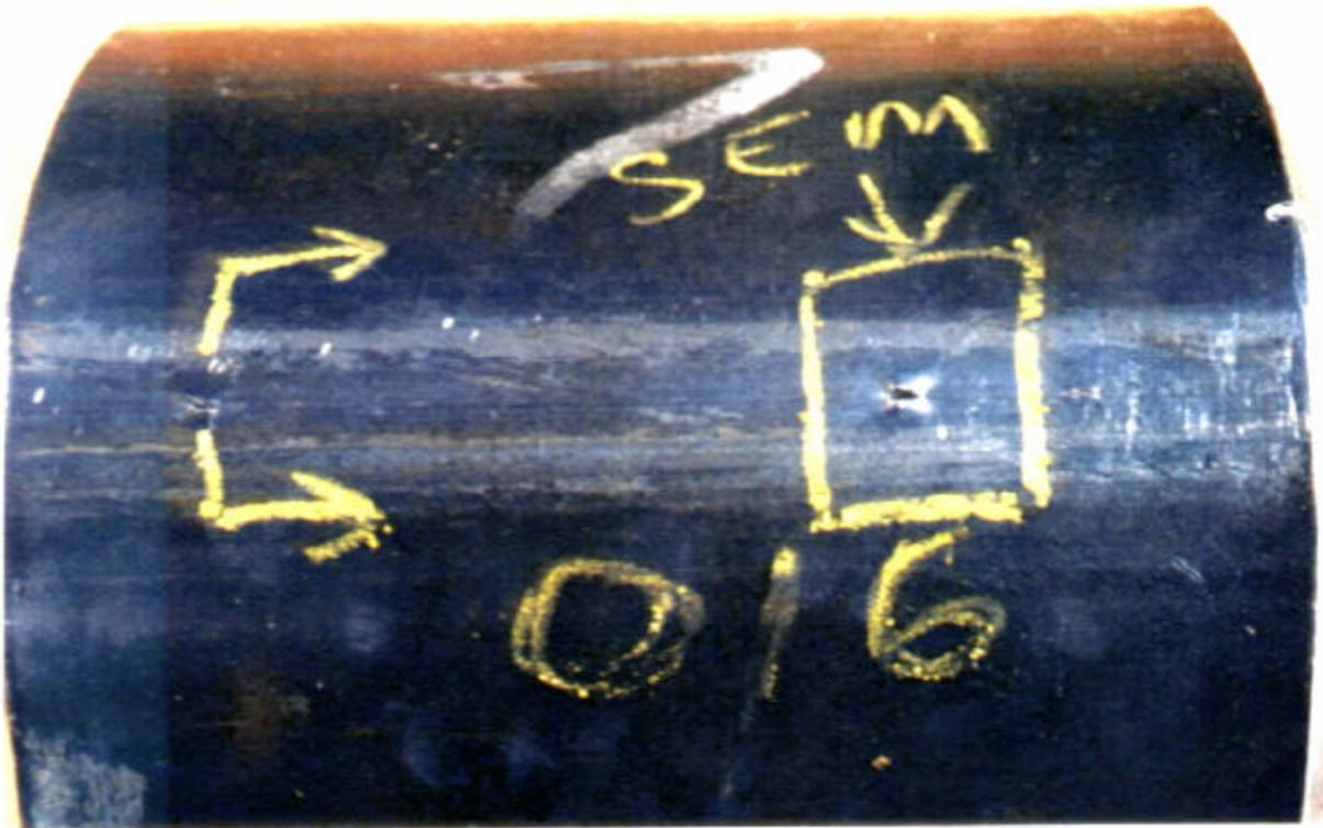
Figure 16 - Typical API flattening test showing split failures in the ERW weld seam
