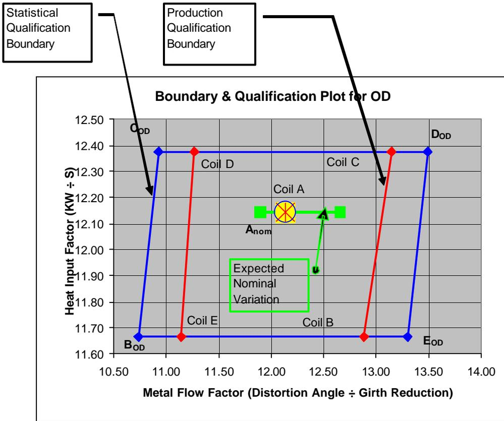
Figure 10 - Qualification boundary chart produced by software using actual production data
