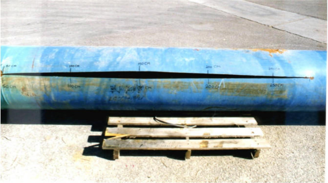
Figure 1 - API 5L X65 20 inch OD and 0.312 inch wall thickness which failed during field hydro-test
