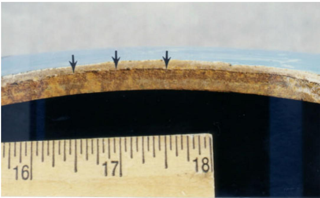
Figure 5 - API 5L X65 20 inch OD and 0.312 inch wall thickness which failed during field hydro-test
