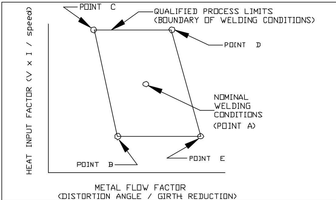
Figure 7 – General qualification boundary for ERW welding conditions
