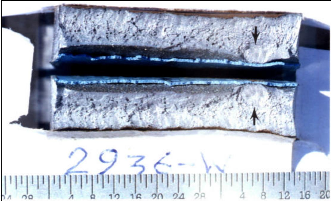
Figure 6 - API 5L X65 20 inch OD and 0.312 inch wall thickness which failed during field hydro-test
