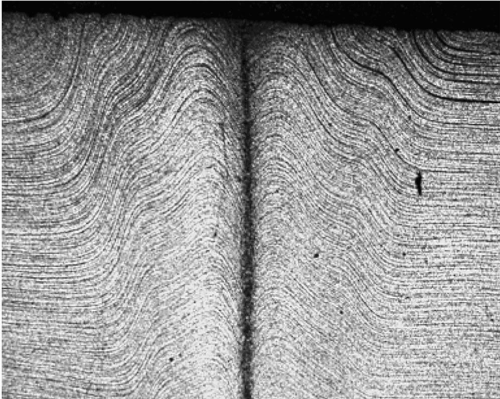
Figure 9 - Typical metal flow pattern for ERW weld seam at OD surface (Picral etch)
