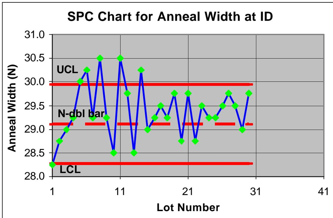
Figure 15 - Typical SPC control chart developed during production
